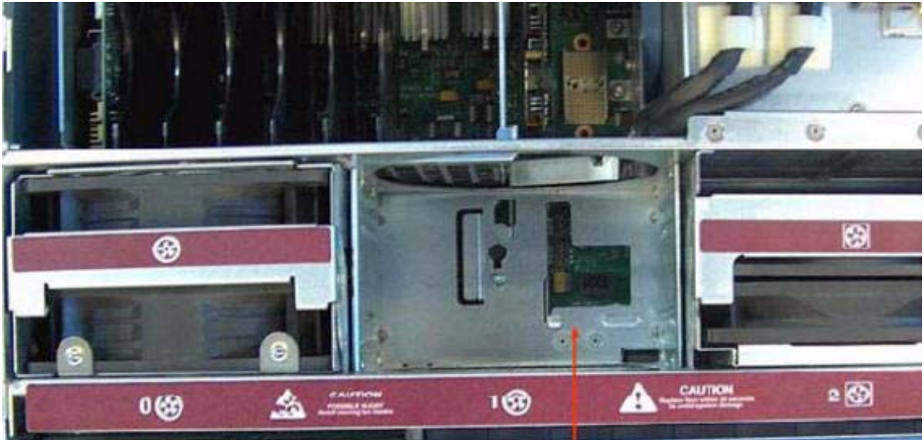
rp44x0 With Top Cover and Center Fan (Fan #1) Removed to Allow Access to I/O Baseboard VGA/CPU Dipswitches
